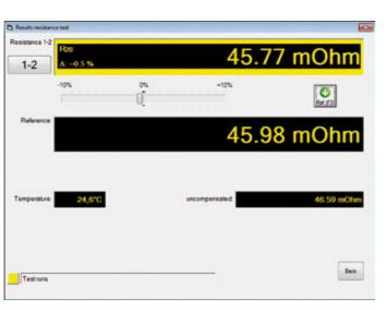
Resistance test e.g. at an air-core coil or bar-to-bar
