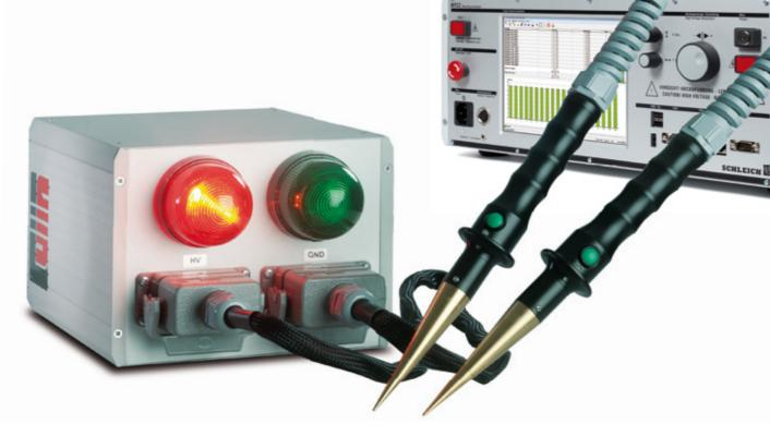
For the armature test an additional armature booster is available for MTC2-testers. This is necessary for testing of larger, low-inductive DC-armatures. With the armature booster the surge current is increased by factor 10, to find short-circuits and insulation faults
