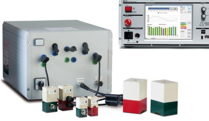
Two test probes are used for the test. They are connected at the test object's exterior above the slots. The first probe (Transceiver) transmits a signal to the test object; the second probe (Receiver) receives the signal. The receipt signal is measured in the MTC2 and the signal strength is displayed on the screen.
